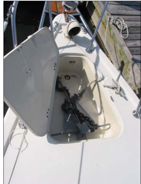
Anchor in anchor well
